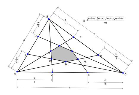
The shaded hexagon is formed by intersecting the lines joining the vertices of the triangle with the trisectors of the opposite sides.
