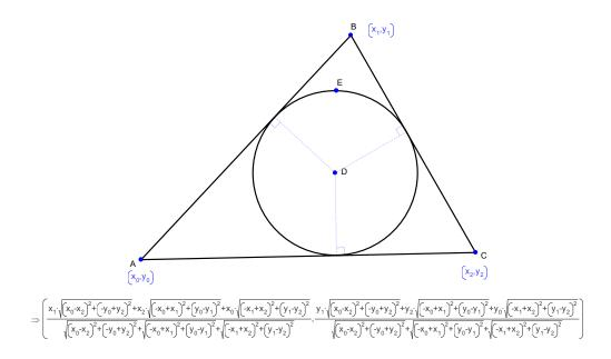
If we let a = |BC|, b=|AC| and c=|AB| and let **A**, **B** and **C** be the position vectors of the points A,B,C then the incircle center is:
